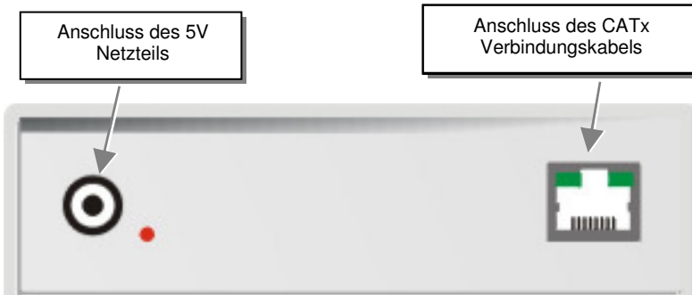
DVXi/ME Media-Extender Typ K466-0C, K466-AC, K467-0C und K467-AC Local/ Remote Unit
