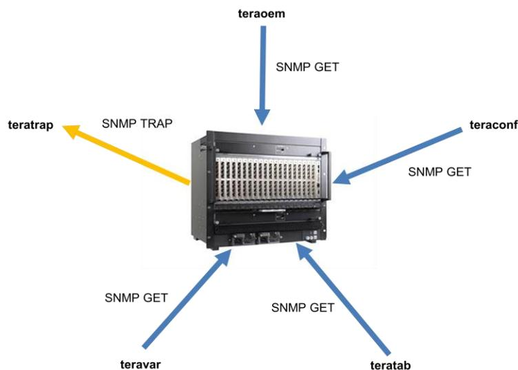
SNMP allows device-specific information to be read from different data areas organized in a tree structure, defined as MIB (Management Information Base). One branch within the MIB tree is officially registered for use by IHSE GmbH (.1.3.6.1.4.1.38034).
