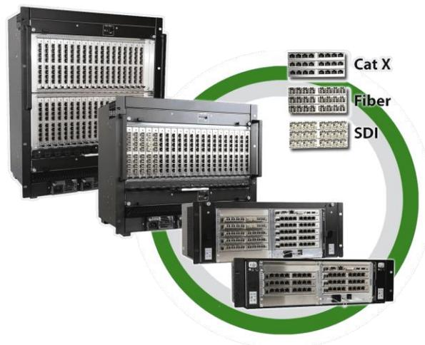
Connections to source computers and display devices are made through CPU and Con Units. A wide variety of these units is available to support all common audio, video USB-HID and USB 2.0/3.0 signal types.
