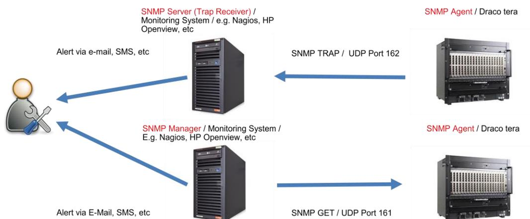
An SNMP agent running in the Draco tera firmware receives a *get* request from a software agent in an SMTP server on UDP port 161 and responds by returning the relevant data. SNMP traps are generated by the SNMP agent and transmitted to the manager on UDP port 162.
