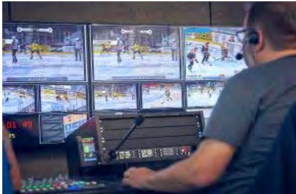
The Finnish league plays more than 450 matches per season, with up to seven games simultaneously. Covering all matches simultaneously (in both HD and UHD) and adding studio production to the program required Streamteam Nordic to build a centralised production hub. The technical solution was designed and implemented by Broadcast Solutions, and it represents the largest broadcast investment in Finland in this millennium.
